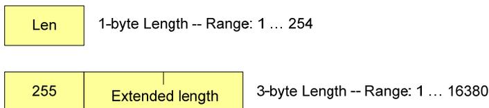
**Figure 3-2: Normal and Extended Length Field.**
