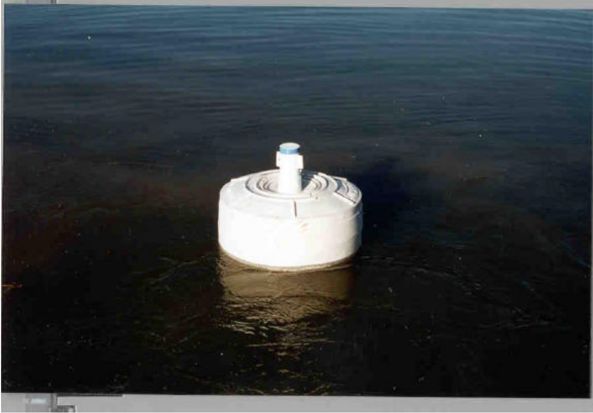
Buoy with Hydrolab's DataSonde 4 collecting data in Newport Back Bay, Ca.
