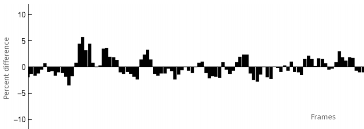
Figure 3 Error associated with randomly varying light, in 100 images of stationary gravel in water.
