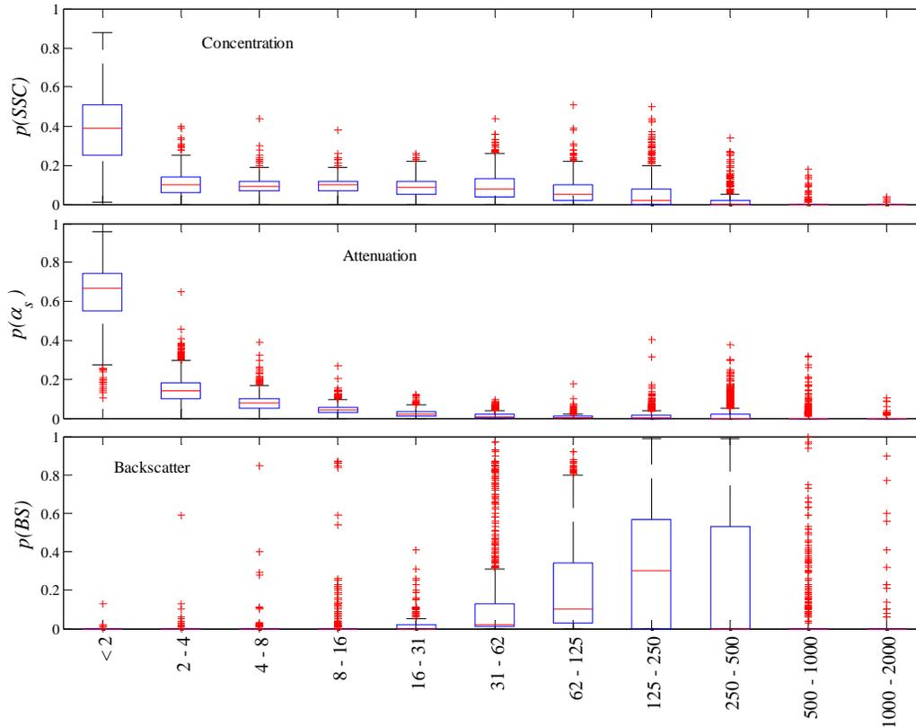
Figure 4 PDFs of concentration (top), attenuation (middle), and backscatter (bottom) for river data used in this study (see Table 1). X-axis particle-size ranges are in microns. Red lines denote median values, box extents are 25<sup>th</sup> and 75<sup>th</sup> percentiles, whiskers lengths are 1.5 times the interquartile range, and points outside this range are red pluses.
