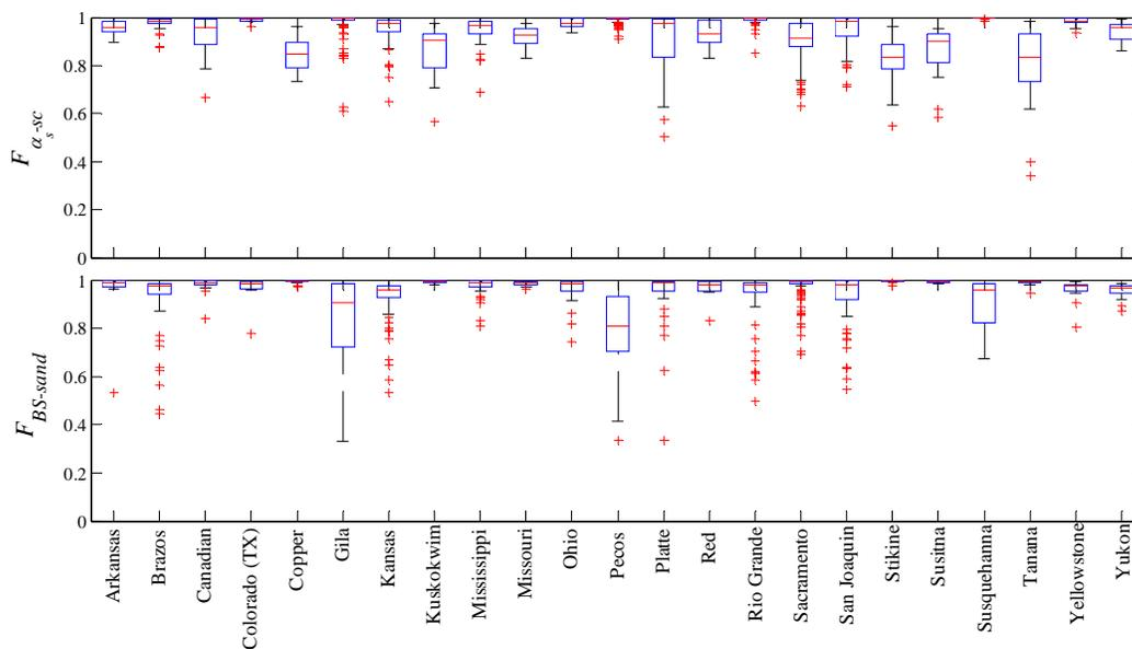
Figure 5 Computed fraction of attenuation due to silt-and-clay (top) and fraction of backscatter due to sand (bottom) for all samples from each river (see table 1).
