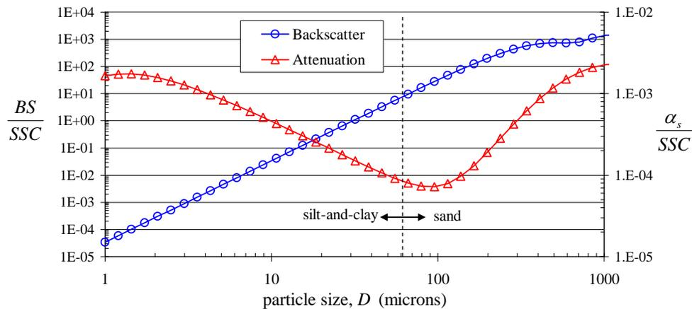
Figure 3 Theoretical relations for backscatter (left axis, blue) and attenuation (right axis, red), for a given suspended-sediment concentration, as a function of particle size (at 1 MHz frequency).
