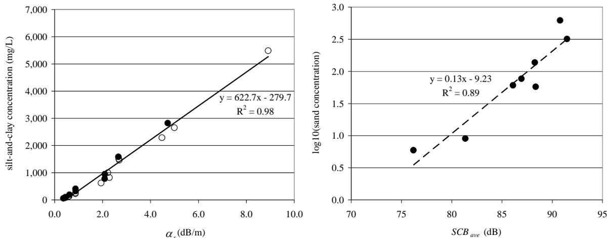
Figure 2 Silt-and-clay concentration versus sediment attenuation (left) and suspended-sand concentration versus backscatter (right) for the Gunnison River, CO.
