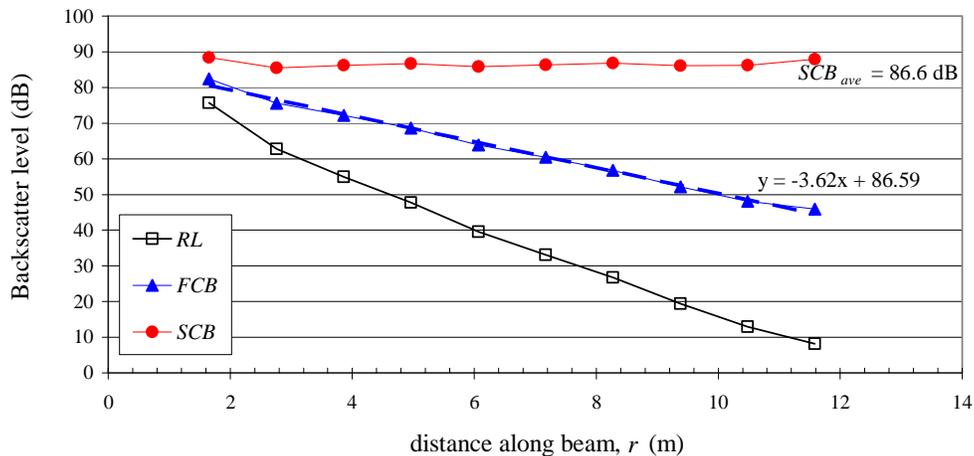
Figure 1 Example of measured and corrected backscatter profiles from the Gunnison River, CO.
