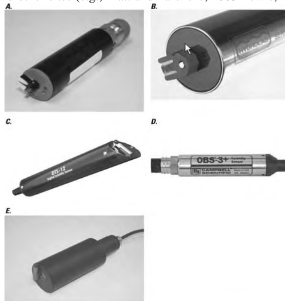
Figure 5. Photographs showing nephelometry sensors: A) YSI model 6136; B) Hydrolab turbidity sensor; and C) Forrest Technology Systems model DTS-12; D) D & A Instrument Company model OBS 3+; and E) Hach OptiQuant with wiper.
