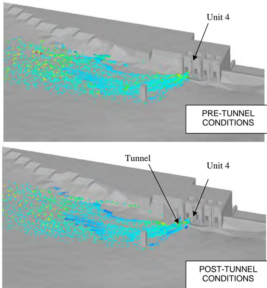
Figure 4 Particle track simulations for the pre-tunnel and baseline conditions.
