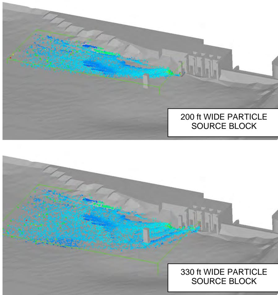
Figure 5 Effect of the source block width on particle tracks.
