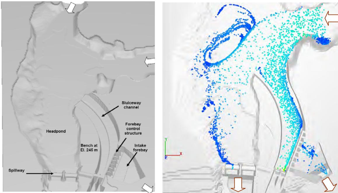
Figure 2 Run-of-river layout and computed particles tracks.
