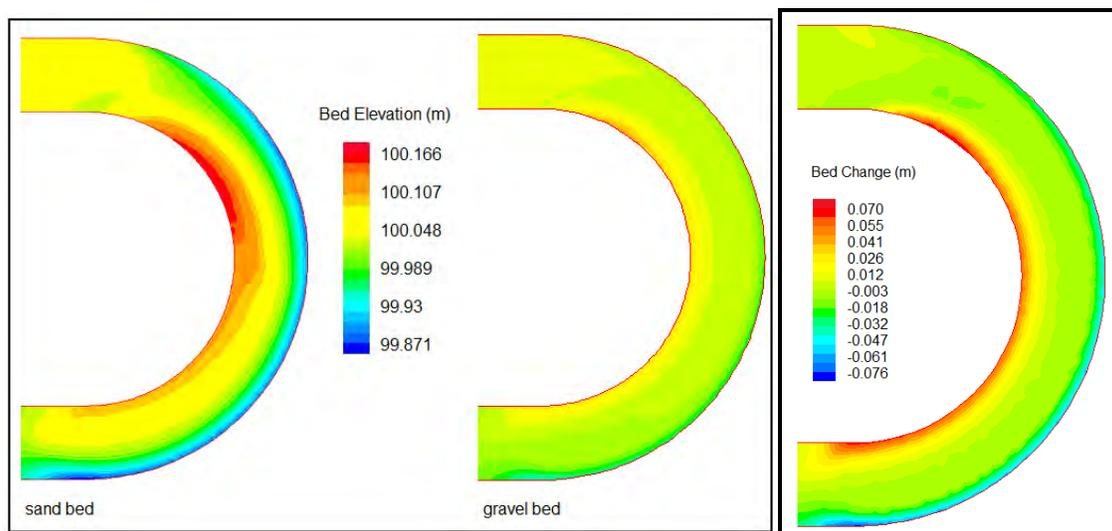
Figure 12. Scour and deposition in a curved flume for sand bed and gravel bed. Bed change shown for gravel bed simulation.
