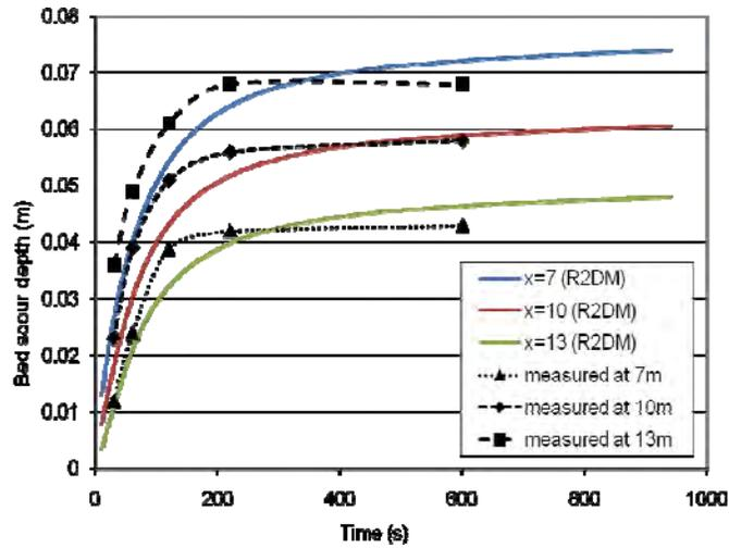
Figure 8. Simulated and measured scour depths for Ashida and Michiue (1971) experiment.
