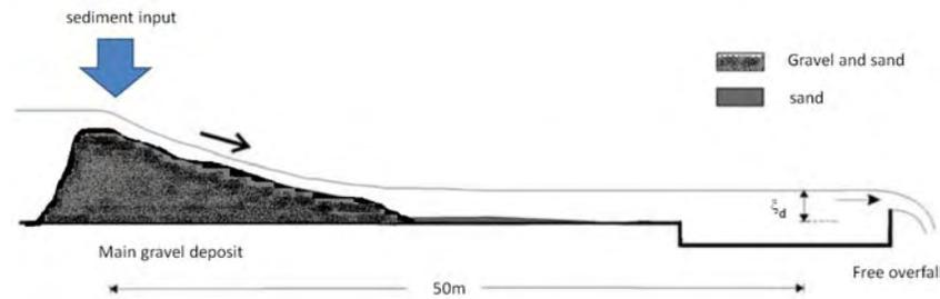
Figure 3. Experiment setup of the SAFL experiments (after Cui, 2007)
