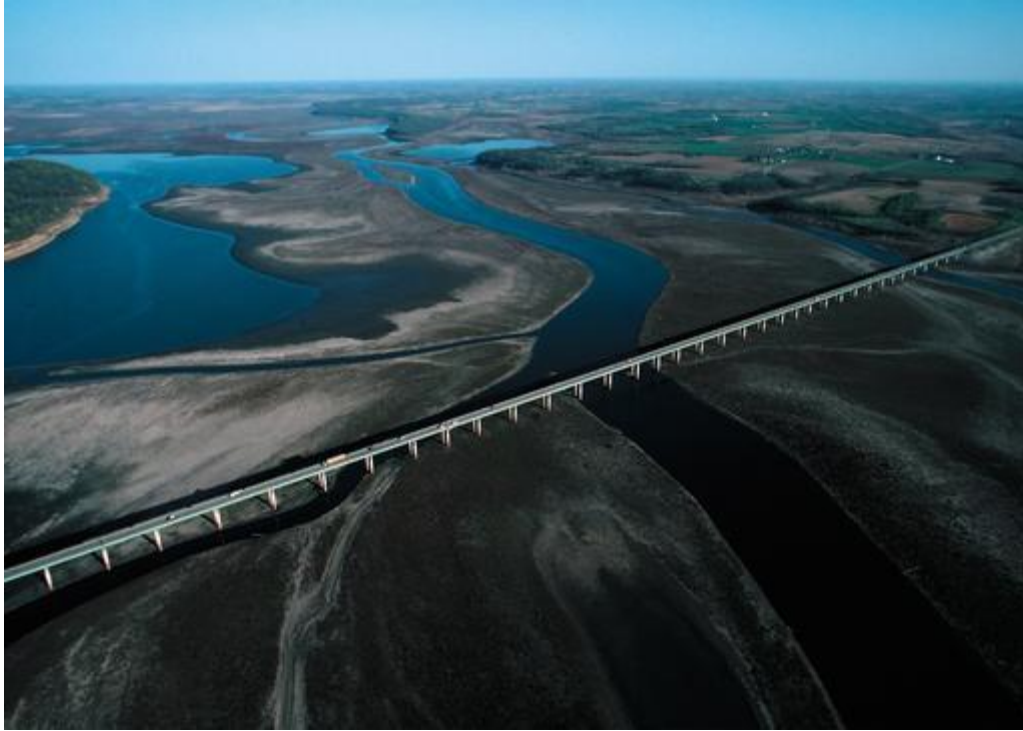
Figure 2. Sediment filling Lake Red Rock in central Iowa at rates much faster than anticipated. (Photo by unknown photographer; Photo courtesy of USDA Natural Resources Conservation Service; Photo by USDA NRCS).
